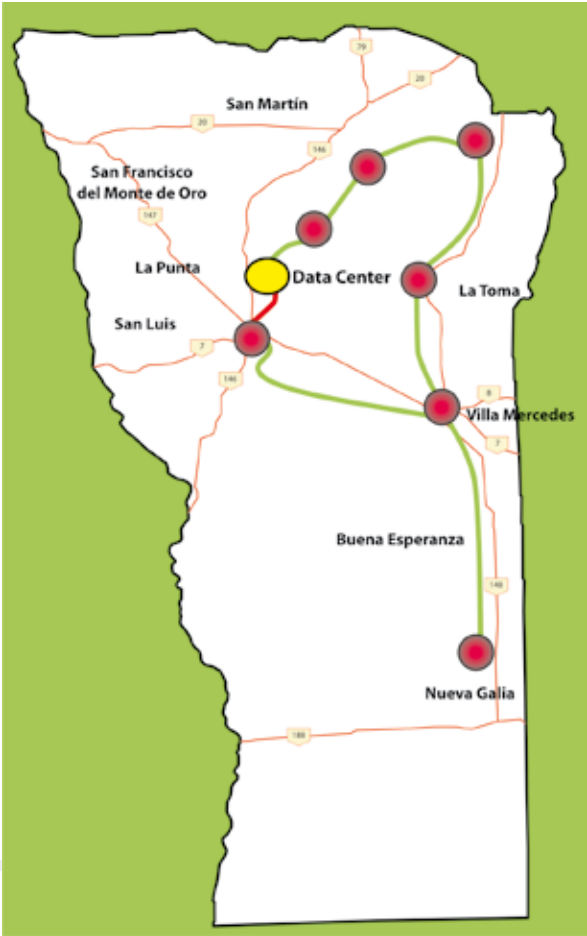
Figura 5: esquema Backbone IP / Figure 5: Backbone IP diagram
