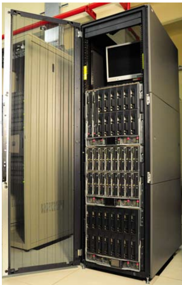
Figura 2: servidores con tecnología Blade / Figure 2: Servers with Blade technology
